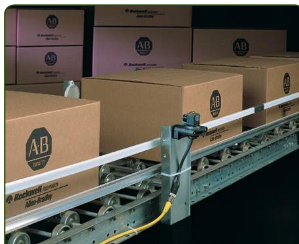
Material handling application – A retroreflective RightSight detecting packages on a conveyor line.
